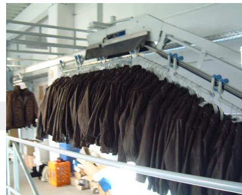
Chain Conveyor (up/down reversible)
