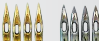
In comparison: GEBEDUR® needle (left) and standard needle (right) after a test
